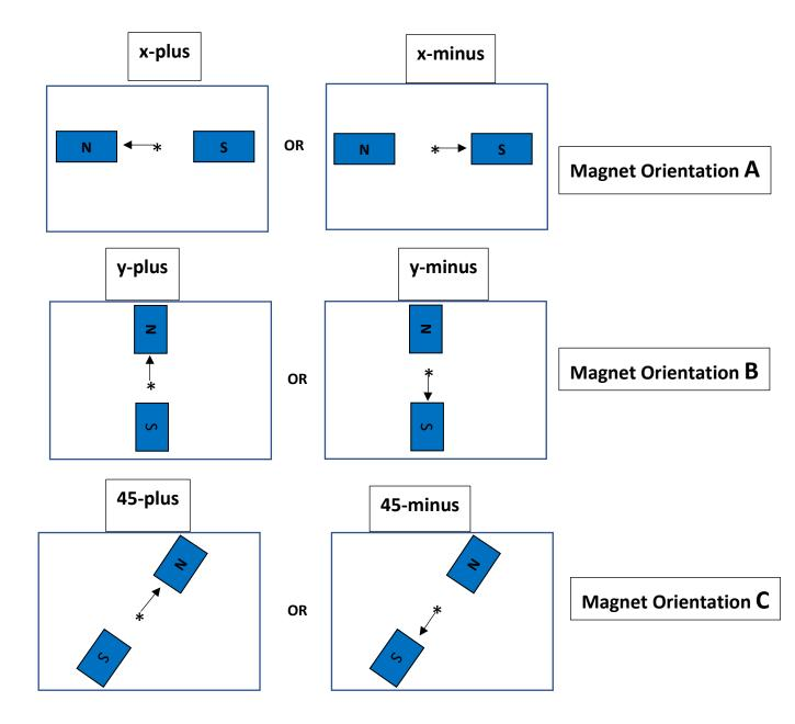
Forward View. The particle goes into the paper (between the magnets)
