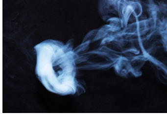
Figure 8: A smoke ring. The core is the center and all around it, there is a vortex flow.
